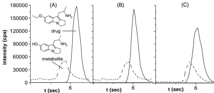
Fig. 4. Separation of drug and phenol metabolite using the dual autosampler setup with mobile phase containing (A) 20%, (B) 25% and (C) 30% acetonitrile in 0.1% formic acid; flow rates: 2.2, 2 and 1.8 ml/min, respectively; column: 2.1 mm  $\times$  10 mm XTerra<sup>TM</sup> RP18 5  $\mu$ m; selected reaction ion current profiles at  $m/z$  259  $\rightarrow$  242 (drug) and  $m/z$  231  $\rightarrow$  214 (metabolite).
