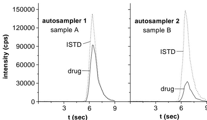
Fig. 3. SRM-LC-MS-MS chromatograms of drug ( $m/z$  259  $\rightarrow$  242) and ISTD ( $m/z$  264  $\rightarrow$  247) in two rat plasma samples analyzed using the dual autosampler setup; column: 2.1 mm  $\times$  10 mm 3.5  $\mu$ m XTerra<sup>TM</sup> RP18 5  $\mu$ m; mobile phase: 25% acetonitrile in 0.1% formic acid; flow rate: 2 ml/min.
