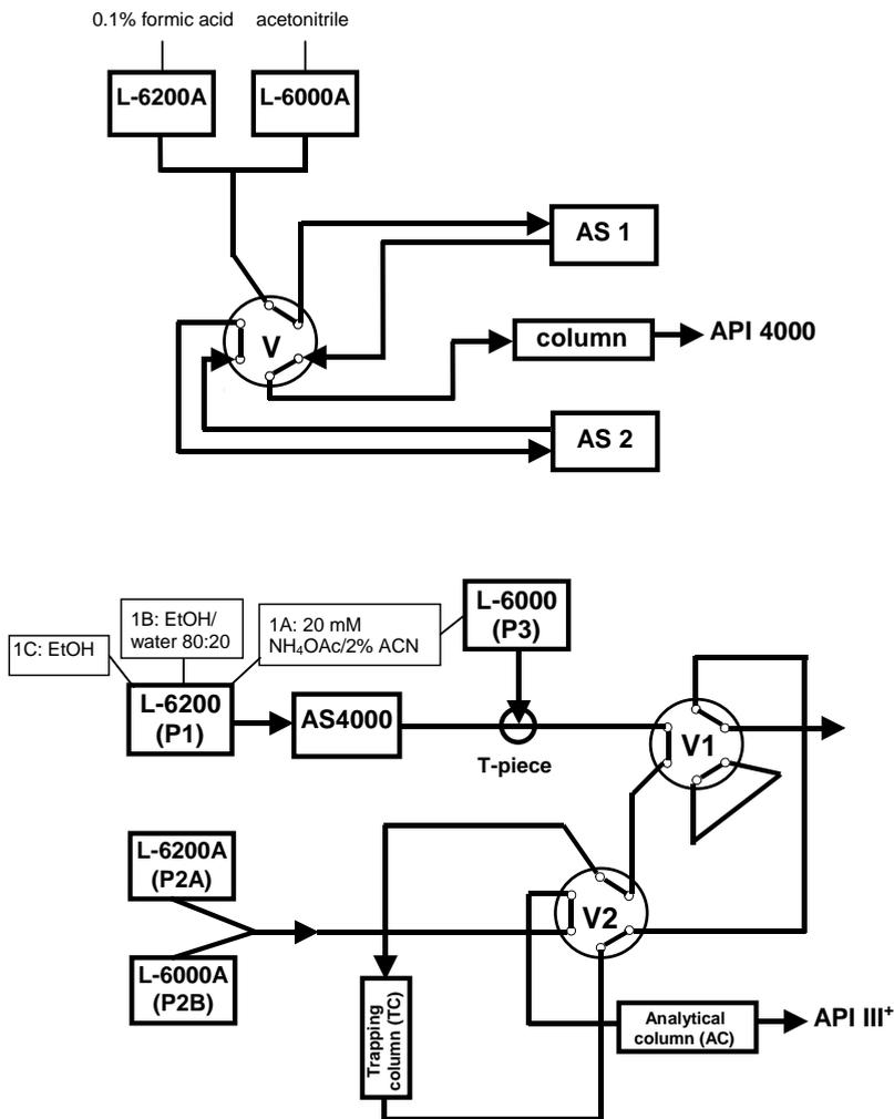
Fig. 1. Schemes of ultra-fast dual autosampler setup (top) and column-switching LC-MS-MS setup (bottom).
