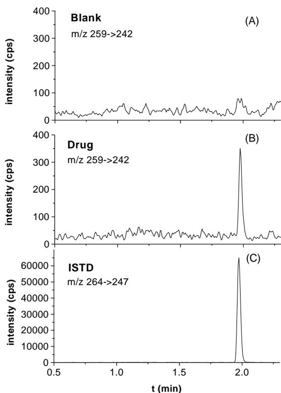
Fig. 5. Column-switching SRM-LC-MS-MS chromatograms of (A) blank plasma at  $m/z$  259  $\rightarrow$  242, (B) drug spiked to plasma at LLOQ 1 ng/ml ( $m/z$  259  $\rightarrow$  242), and (C) internal standard ( $m/z$  264  $\rightarrow$  247); for conditions, see Table 1.
