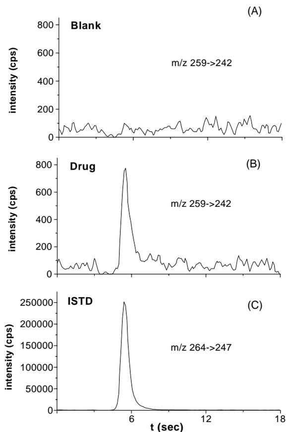
Fig. 2. SRM-LC-MS-MS chromatograms of (A) blank plasma at  $m/z$  259  $\rightarrow$  242, (B) drug spiked to plasma at LLOQ 1 ng/ml ( $m/z$  259  $\rightarrow$  242), and (C) internal standard ( $m/z$  264  $\rightarrow$  247); column: 2.1 mm  $\times$  10 mm 5  $\mu$ m XTerra<sup>TM</sup> RP18; mobile phase: 25% acetonitrile in 0.1% formic acid; flow rate: 2 ml/min.
